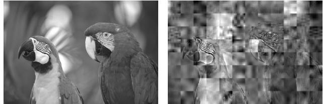
Figure 3. Original encoded image (left, error rate = 10^{-16} , PSNR = 40 dB) and the same image naively stored in unoptimized and untuned approximate cells, with unacceptable quality degradation (right, error rate = 10^{-3} , PSNR = 18 dB).
