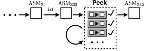
**Figure 1. Peek Backend** CompCert produces code in  $\text{ASM}_{\mathbb{Z}}$ . We prove a forward simulation to establish that a program will have equivalent behavior under  $\text{ASM}_{\mathbb{Z}32}$ . Peek repeatedly applies peephole optimizations from a set of verified rewrites to the code.
