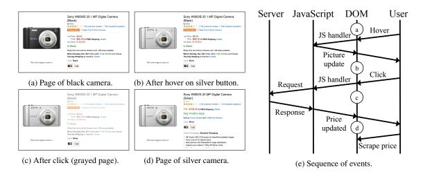
Figure 1: Amazon price scraping interaction. Each circle in (e) corresponds to a webpage state shown in (a-d). Note that hovering over the silver option instantly displays the silver camera picture but not its price. Only after the click does the page request the silver price from the server and overlays to gray. The response updates the price and removes the gray overlay.
