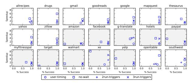
Figure 7: Success rate v. speedup on a set of benchmarks. Benchmarks with shaded backgrounds require synchronization.
